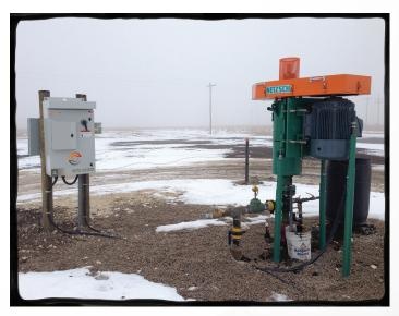
30 HP installation shown. The Roto-Armor VFD has highly accurate motor control to carefully regulate applied motor torque, eliminating torque overshoot and its associated problems.
