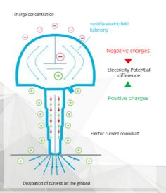
Variable electric field balancing device.
